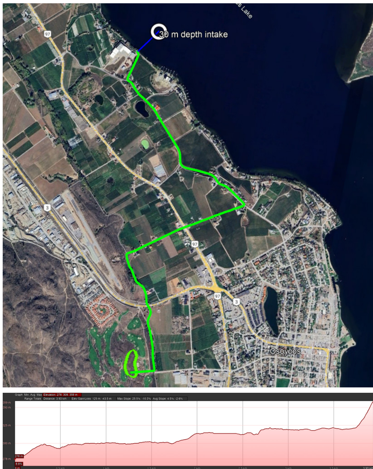
Figure 12 Plan and Profile of Proposed Raw Water Pipeline Connecting Osoyoos Lake Intake to Treatment Plant at the Reservoir Site
